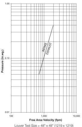
Pressure loss tested in accordance with Figure 5.5 of AMCA Standard 500-L. Data corrected to standard air density.
